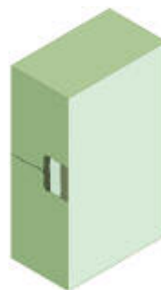
Figure 4: Apply Krystol T1 Slurry Coat
